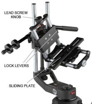
6) Adjust the L-Shaped camera support up and down to position the center of gravity of the camera on the tilt axis of the head. To do this, release the two lock levers, tilt the camera 90 degrees so that it is pointing straight down, then adjust the lead screw until the camera stays balanced when you let go of the pan bar. The camera should remain balanced at any angle through the 360 degree tilt range.
